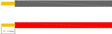
2. Insert the black wire to blue clamp, red wire to red clamp, and fasten screws tightly, see below:
